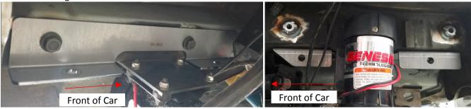
*Winning with Personal Service since 2001* Rear Fascia Support Installation Guide, Rev 1.1, 5-30-18 2.4 Install Fascia Support with four M10x1.5x25 Flange Bolts (30ft-lbs) to the Upper Weld Bungs and the Fascia Support Frame Clip.
