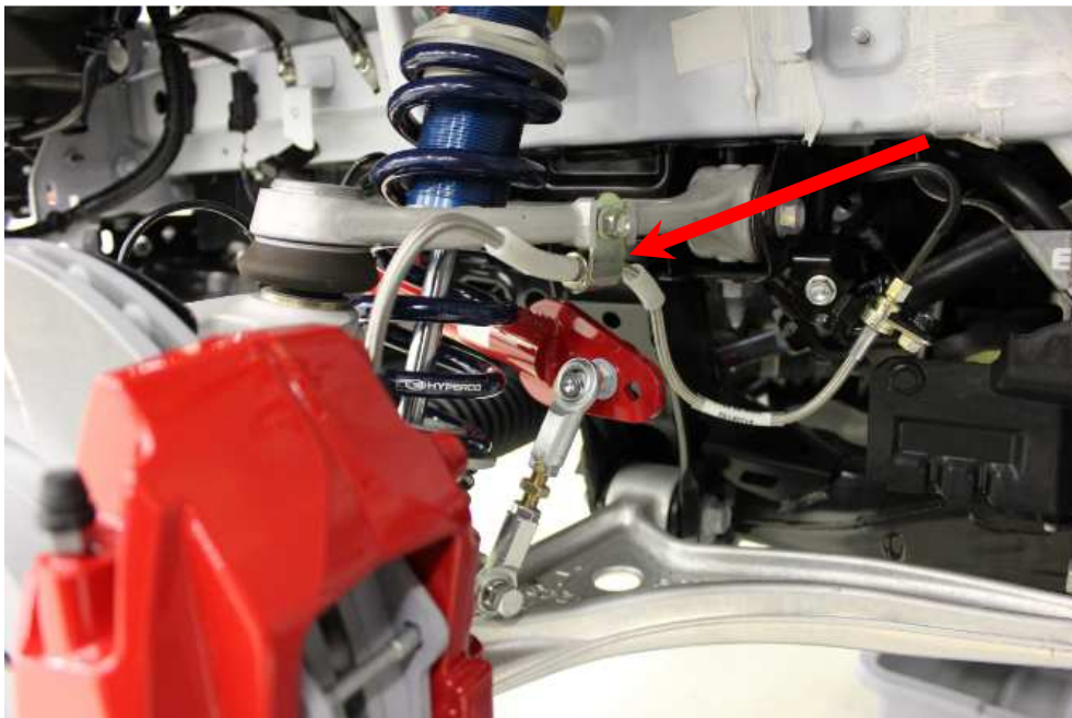
Figure 1. Brake Line Mounted on Bottom of Control Arm. ← Incorrect brake hose mounting
