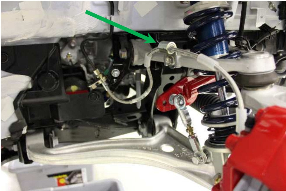
Figure 2. Brake Line Mounted on Top of Control Arm. ← Proper brake hose mounting
