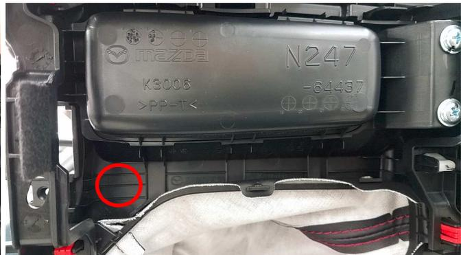
3. Run wires under center console up to steering column and plug the Pit Speed Selector harness into Channel 05 of the AiM MXL2 analog inputs, secure wires with zip ties.
