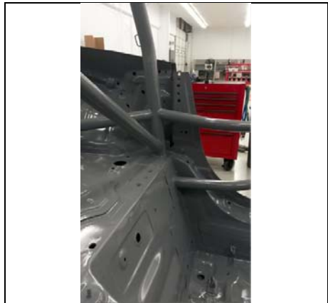
PHOTO 4 MAIN ROLLBAR TO FLOOR ATTACHMENT
