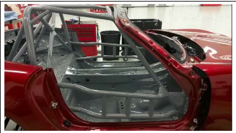
PHOTO 5 REAR BACKSTAY TO BODY ATTACHMENT
