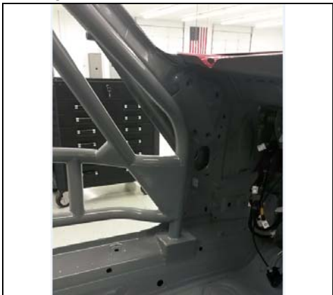
PHOTO 6 FRONT ROLLBAR TO FLOOR ATTACHMENT
