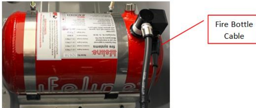
Figure 3. Fire Bottle Cable, Trunk.
