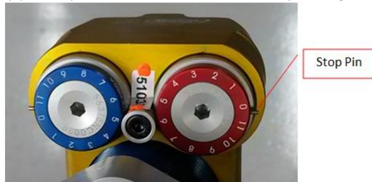
Figure 10: Damper Valve with Seal. 5 Compression, 6 Rebound Shown
