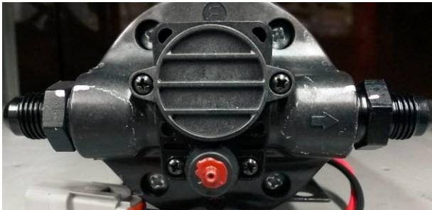
Figure 15: Transmission and Differential Cooling Pump
