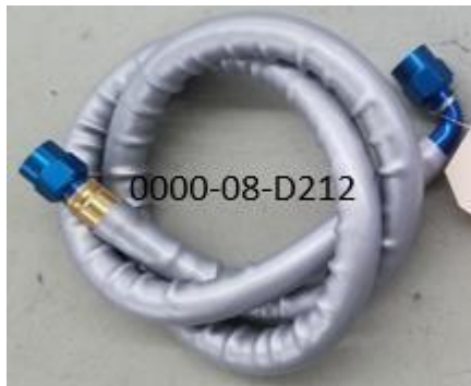
Dash 6 Oil Line, Trans-Cooler to Pump-ND2 0000-08-D212
