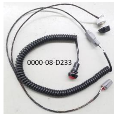
Speed Limiter, Pit Lane-ND2 0000-08-D233
