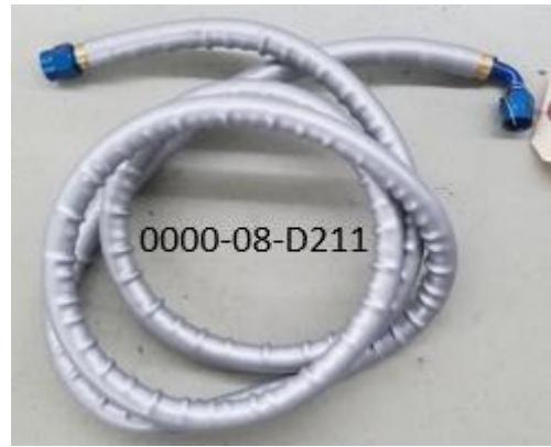
Dash 6 Oil Line, Trans-Filter to Cooler-ND2 0000-08-D211
