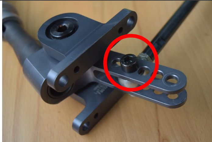
The only Homologated Shift Linkage position, is the second mounting hole from the top, as pictured above. No exceptions.
