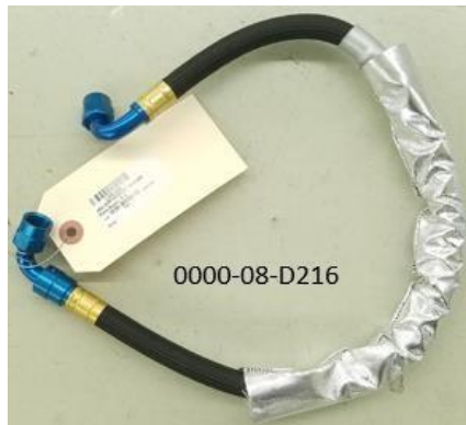
Dash 6 Oil Line, Diff-Cooler to Pump-ND2 0000-08-D216
