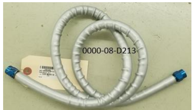
Dash 6 Oil Line, Trans-Pump to Housing – ND2 0000-08-D213- NON- SADEV
