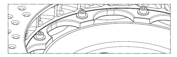
INSTALL DISC MOUNTING HARDWARE AS SHOWN. SCREWS ARE DELIVERED WITH THREAD LOCK COMPOUND ALREADY APPLIED. SCREWS ARE TORQUED TO 7 Nm (62 in-1bs). THE FASTENERS WILL NOT FIRMLY CLAMP THE BELL AND DISC TOGETHER, THEREFORE, THE BUSHINGS WILL SEEM TO BE SLIGHTLY LOOSE.
